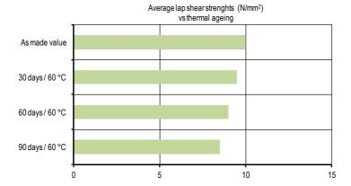
The tests have been carried out at 20 °C on steel to steel joints, which have been aged at 60 °C.
