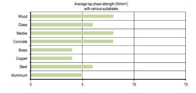
The tests have been conducted at  $20^{\circ}$ C on metal to metal joints, which have been hardened for 48 hours at  $20^{\circ}$ C.
