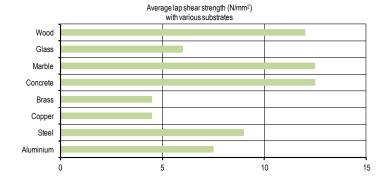
The tests have been conducted at 20°C on metal to metal joints, which have been hardened for 48 hours at 20°C.
