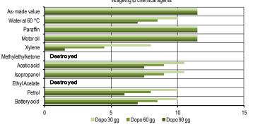
If not otherwise specified, the tests have been carried out at 20 °C after immersion for 30, 60 and 90 days at 20 °C on steel to steel joints which have been hardened for 48 hours at 20 °C.
