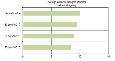
The tests have been carried out at 20 °C on steel to steel joints, which have been aged at 60 °C.
