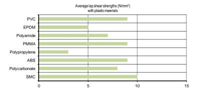
The tests have been conducted at 20°C on plastic to plastic joints, which have been hardened for 48 hours at 20°C.
