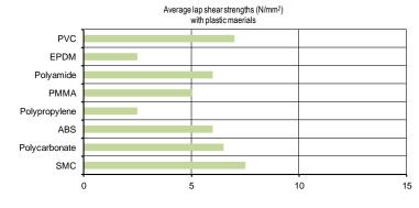
The tests have been conducted at  $20^{\circ}$ C on plastic to plastic joints, which have been hardened for 48 hours at  $20^{\circ}$ C.
