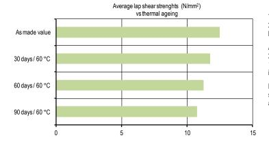
The tests have been carried out at 20  $^\circ\text{C}$  on steel to steel joints, which have been aged at 60  $^\circ\text{C}.$
