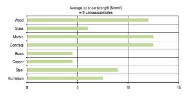
The tests have been conducted at  $20^{\circ}$ C on metal to metal joints, which have been hardened for 48 hours at  $20^{\circ}$ C.
