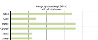
The tests have been conducted at 20°C on metal to metal joints, which have been hardened for 48 hours at 20°C.
