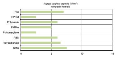
The tests have been conducted at 20°C on plastic to plastic joints, which have been hardened for 48 hours at 20°C.
