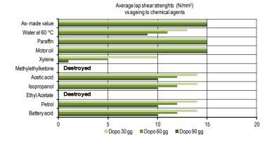
If not otherwise specified, the tests have been carried out at 20  $^{\circ}$ C after immersion for 30, 60 and 90 days at 20  $^{\circ}$ C on steel to steel joints which have been hardened for 48 hours at 20  $^{\circ}$ C
