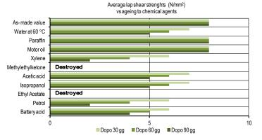
If not otherwise specified, the tests have been carried out at 20 °C after immersion for 30, 60 and 90 days at 20 °C on steel to steel joints which have been hardened for 48 hours at 20 °C.
